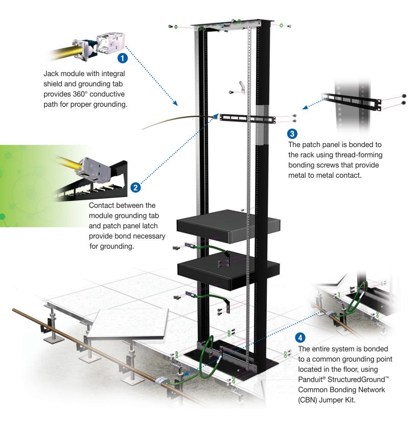
• Integrated grounding and bonding provides an easy to install shielded cabling system
